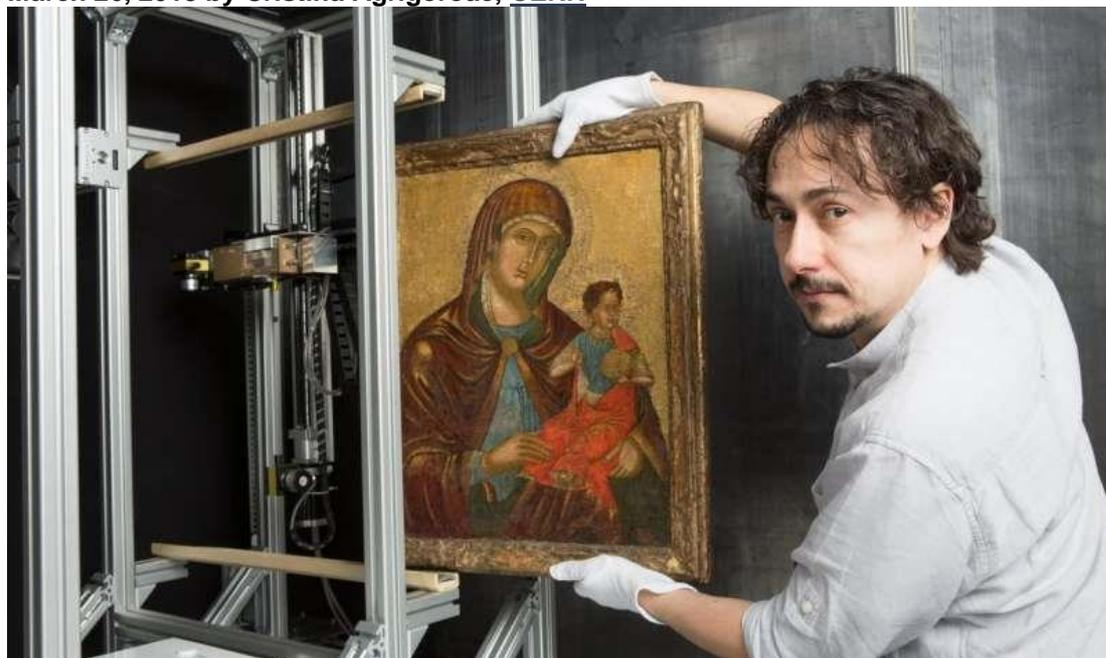
Slotting a painting into the X-ray scanner, which will analyse it at a high resolution. Credit: InsightArt s.r.o.
