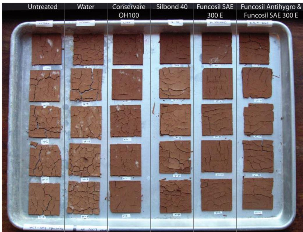
Fig. 7. Samples before wet-dry cycling viewed from above. Each column contains samples treated with the same consolidant. From left to right they are: untreated (control), water, Conservare OH100, Silbond 40 with ethanol in a 1:1 solution by volume, Funcosil SAE 300E, and Funcosil Antihygro pre-treatment with Funcosil SAE 300E.
