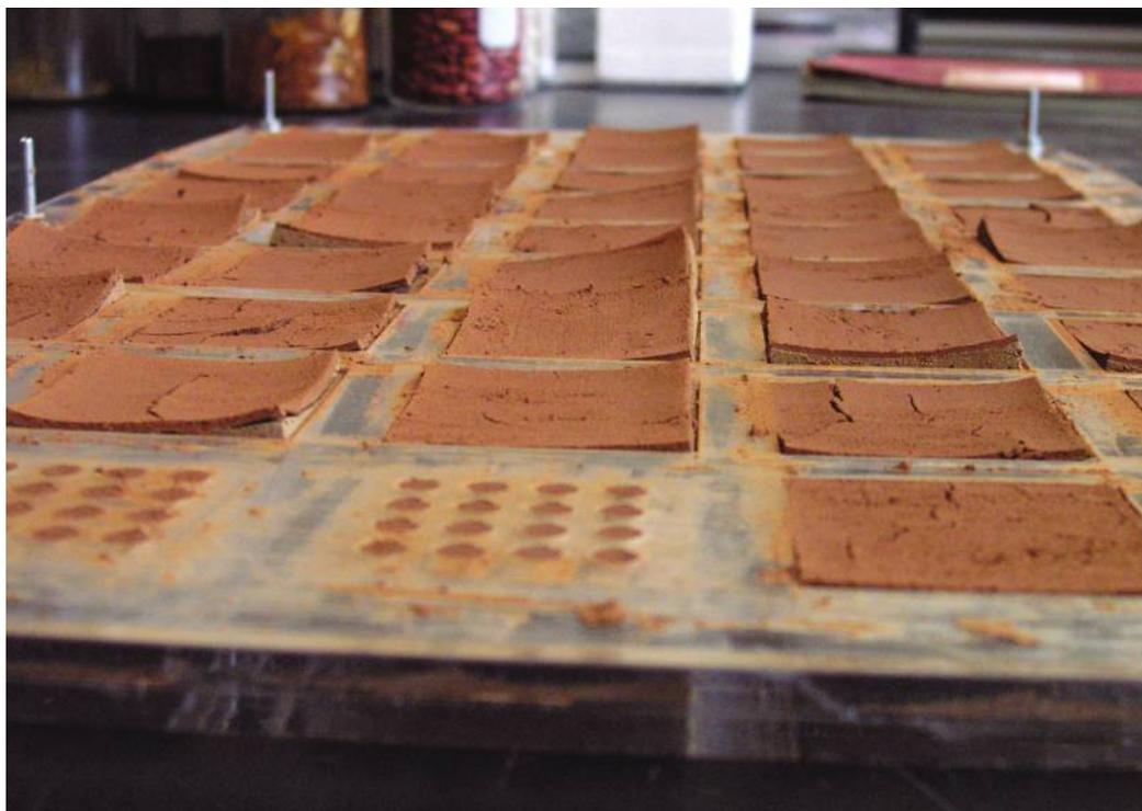
Fig. 1. Planar distortion of samples after drying. Samples were prepared in a laser-cut acrylic mold for optimal control of their dimensions. Two layers were applied—a 6 mm-thick plaster, topped by 1.5 mm of wash layer. A second set of samples was produced with only the thin wash layer.
