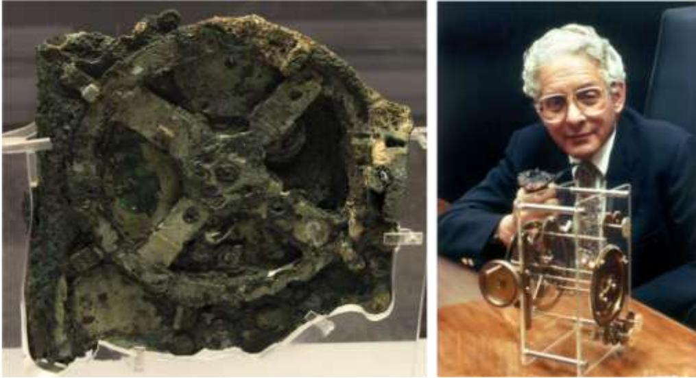
The Antikythera mechanism in its corroded state and a modern replica. Courtesy of Wikimedia Commons.
