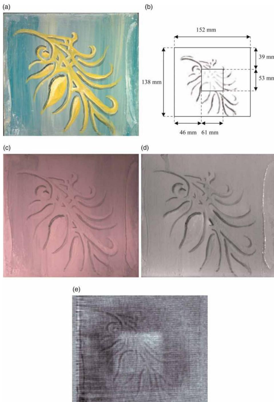
FIG. 3. The self-made sample, mimicking a panel painting. Oil, tempera, wood. (a) The general image of the sample, (b) the scheme of the defect location, (c) near-infrared image of the sample (made with a silicon CCD detector, spectral band: 0.7–1.1  $\mu\text{m}$ ), (d) SWIR image of the sample (made with InGaAs detector, spectral band: 0.9–1.7  $\mu\text{m}$ ), (e) thermographic image collected from the sample (MWIR spectral band, 3–5  $\mu\text{m}$ , principal component processing applied).
