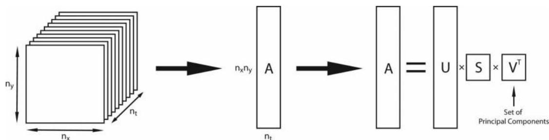
FIG. 1. An explanation of PCT data processing. The 3D array of raw thermographic data is first converted into a 2D array, which is then converted into a product of three matrices. Matrix  $V$  contains a set of principal components, representing the “temperature trends.”
