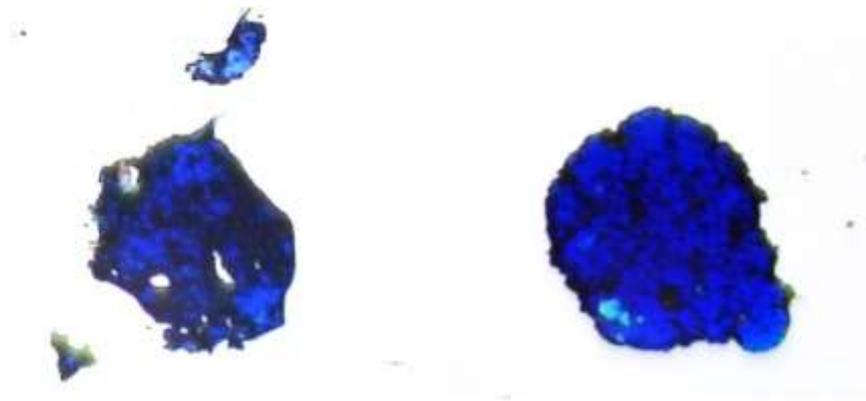
**Figure 1.** (Left) Acrylic Prussian blue hue; (Right) Oil based Prussian blue.
